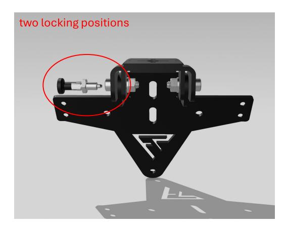
Mount the locking pin on the right side for one locking position, or on the other side for two locking positions.
