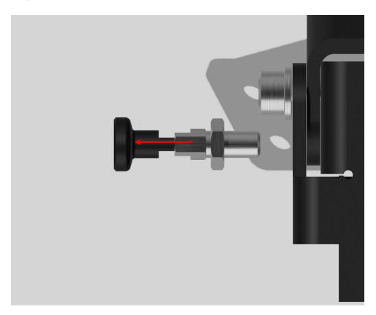
Apply a medium-strength threadlocker (e.g., Loctite) to the locking pin and pre-load it before screwing it in.
